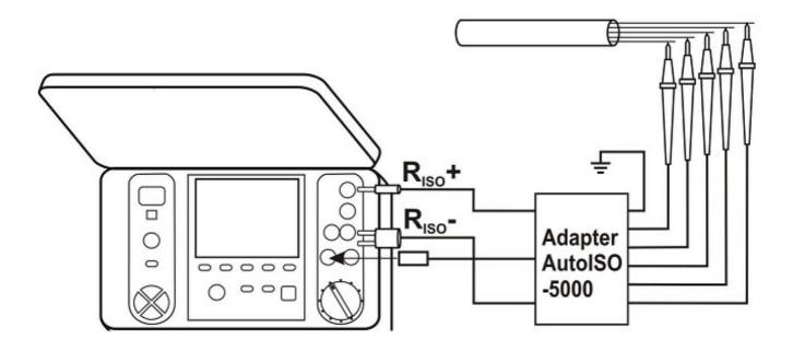
The <u>AutoISO-5000</u> adapter for Sonel Insulation Meters vastly simplifies insulation testing of multi-conductor cables, and cuts the time to test by 50 - 75%.
