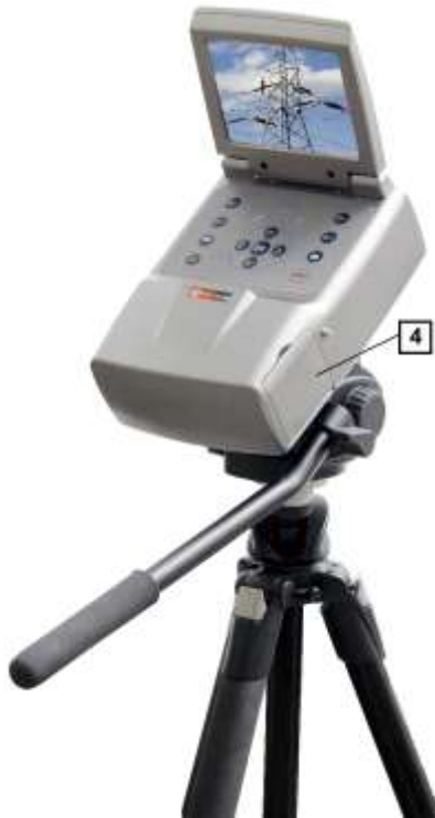
Fig. 12 UV-260 mounted on a tripod.
