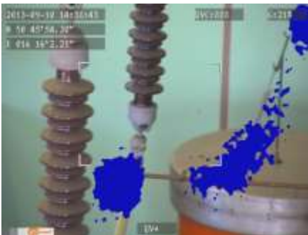
Fig. 3, 4. Corona discharge in laboratory conditions.
