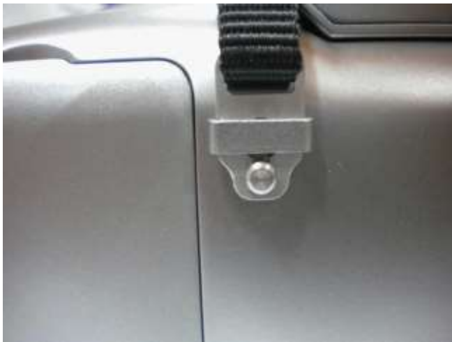
Fig. 13. Fixing strap to the holders.
