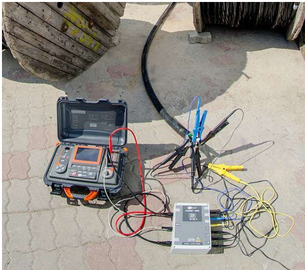
AUTOISO 5000 Adapter for testing multi-conductor cables
